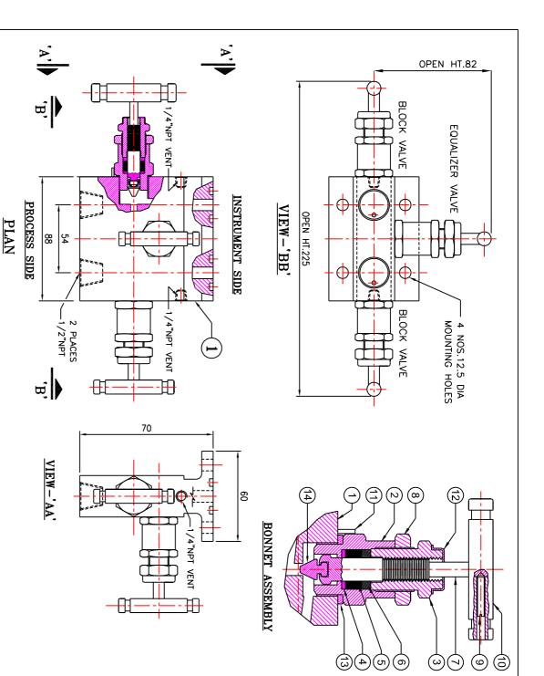
PANAM 3 VALVE MANIFOLD 1-TYPE PIPE TO FLANGE CONNECTION DESIGN FOR CONNECTING SYSTEM IMPULSE LINES AND TRANSMITTERS. THIS MANIFOLD CONSISTS TO 1/2" NPT FEMALE CONNECTIONS ON 54mm.(2-1/8") CENTERS AND OF ONE EQUILIZER VALVE AND TWO BLOCK VALVES.1/4"NPT PURGE CONNECTIONS ARE OPTIONAL.
